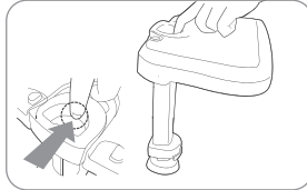
Pushing the button (protrusion) of the Foot Plate hole inside, join the Foot Plate and the Height Control Bar
